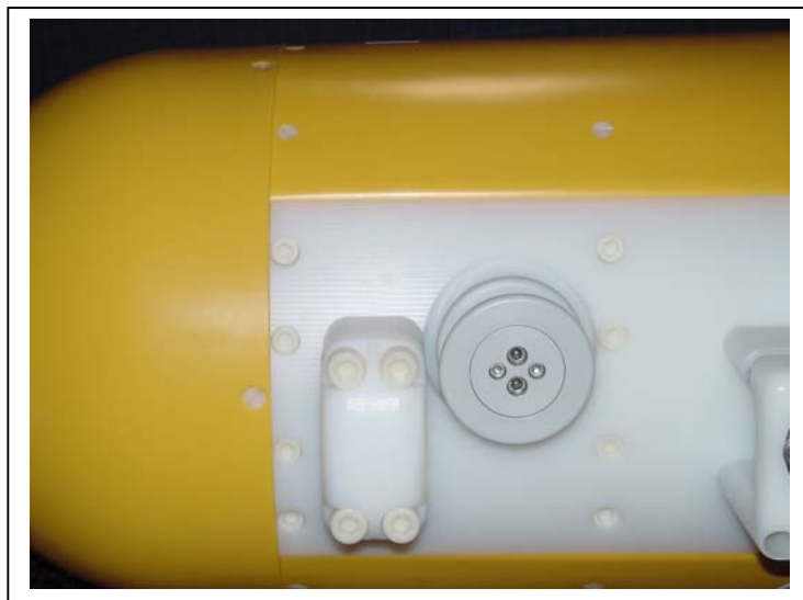
Figure 2-6: Cable Retainer and Guide Wheel
