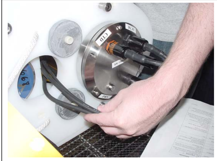
Figure 2-8: Gathering Excess Cable Length
