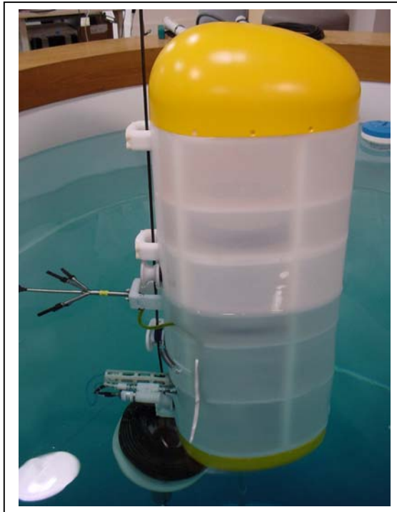
Figure N-1: MMP with Battery Housing Glass Sphere Extension
