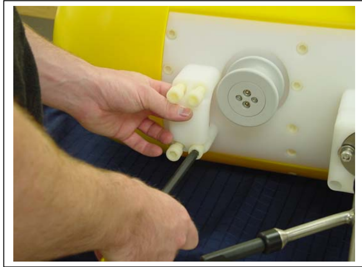
Figure 6-4: Removing the Cable Retainers
