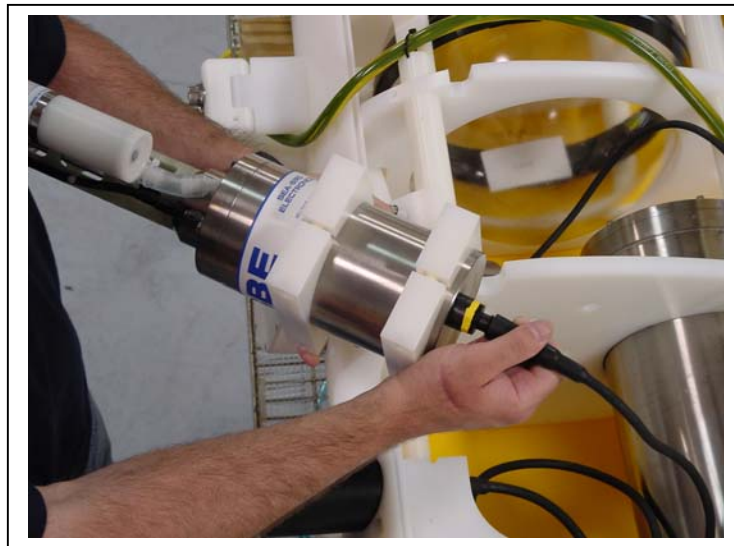
Figure L-15: Unplugging the Bulkhead Connector
