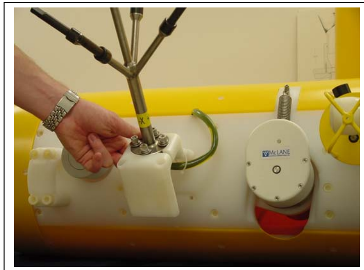
Figure 6-3: Loosening the ACM Hinged Bracket
