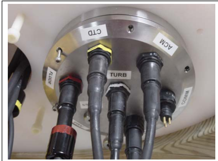
Figure I-2: MMP End Cap with Sensor Connections
