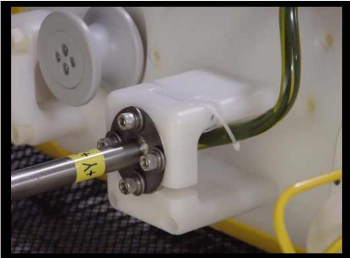
Figure 2-15: Mounting the ACM Sting
