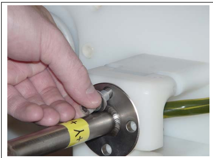
Figure 2-14: Swinging the ACM Sting Out of the Way
