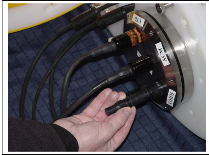
Figure 6-2: Connecting the Battery
