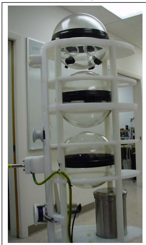
Figure N-18: Glass Battery Housing Sphere Installed
