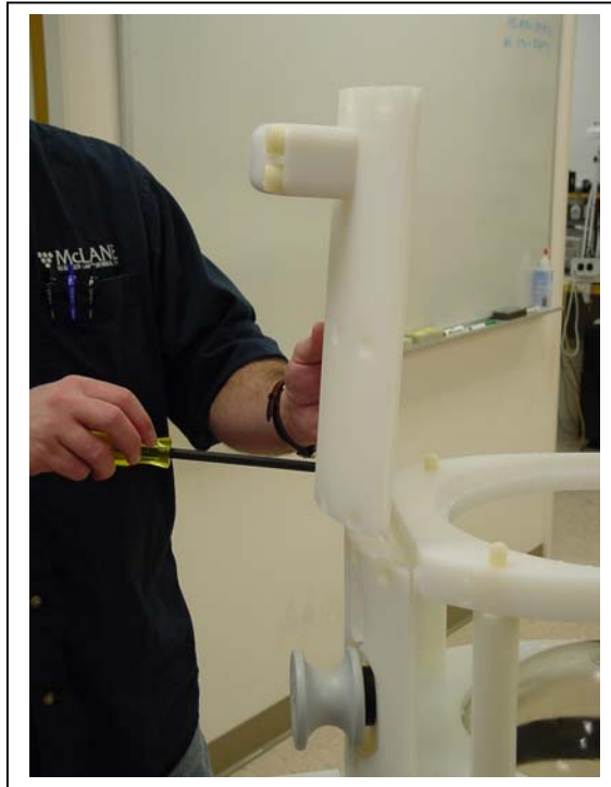
Figure N-11: Installing Front Panel Extension
