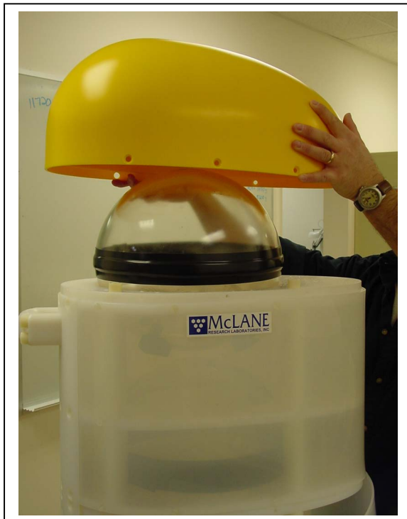
Figure N-5: Removing Top Cap
