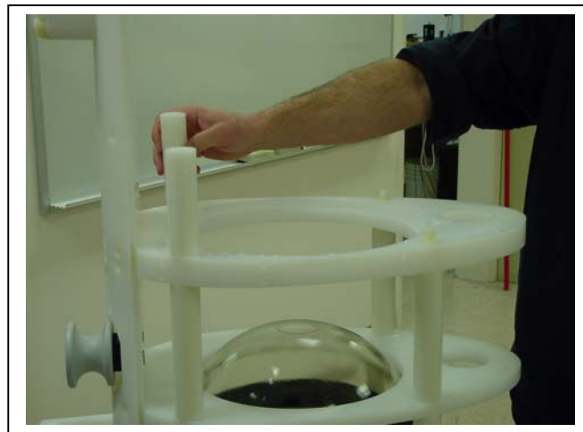
Figure N-12: Installing Spacer Legs with Studs
