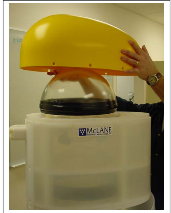
Figure N-22: Reinstalling Top Cap
