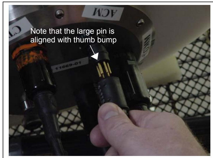
Figure 4-1: Cable Connector Alignment
