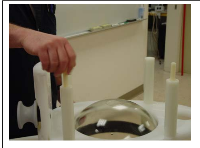
Figure N-9: Installing Nylon Studs
