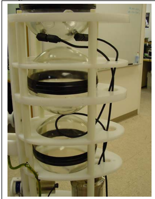
Figure N-19: Routed and Connected Cable
