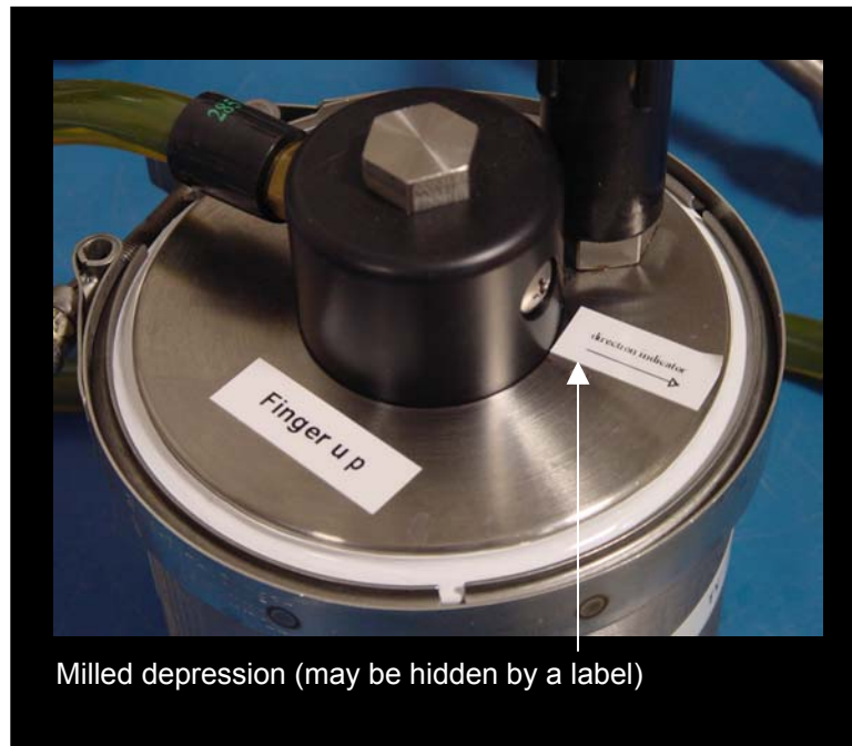
Figure 2-16: Correct Positioning of ACM Electronics Housing
