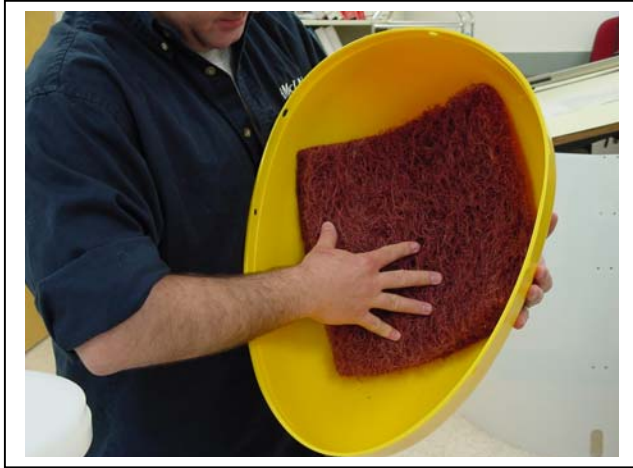
Figure N-21: Reinstalling Horsehair
