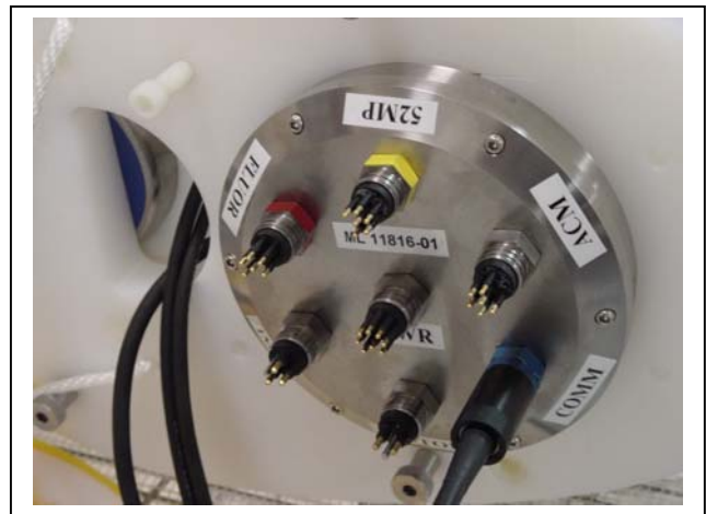
Figure N-24: Color-Coding on End Cap
