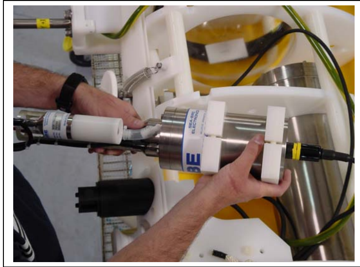
Figure L-14: Lifting the CTD from the Sensor Mount
