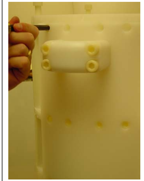
Figure N-16: Installing and Tightening Cap Screws on Front Panel
