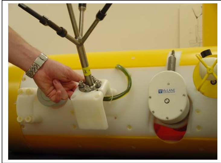
Figure 2-13: Securing the ACM Sting Cable
