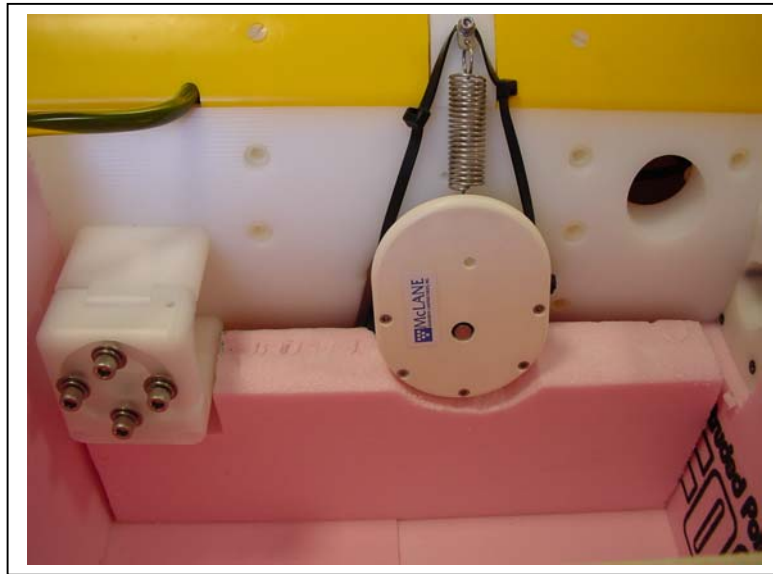
Figure 4-3: Stabilizing the Motor in the Crate
