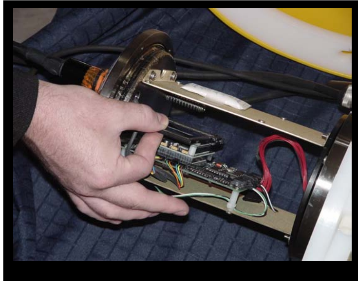
Figure 8-1: Flash Card Removal
