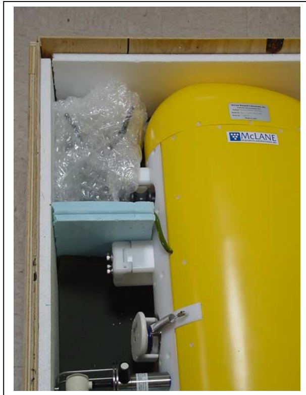
Figure 4-2: Fitting the MMP in the Crate
