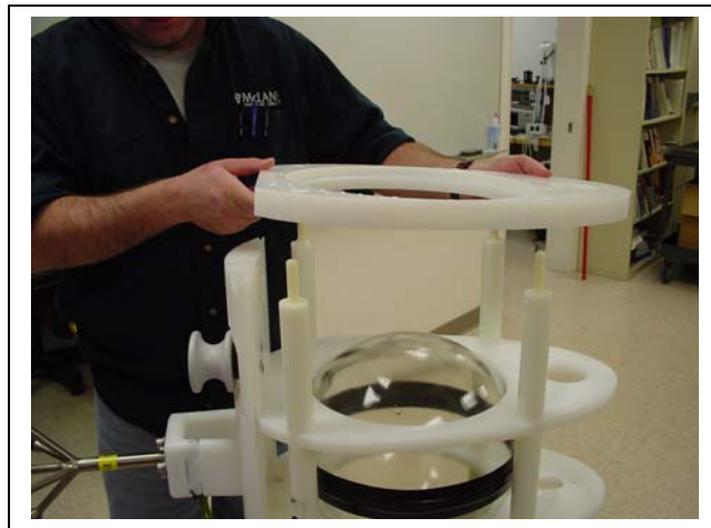
Figure N-10: Installing M3100A Extension Plate
